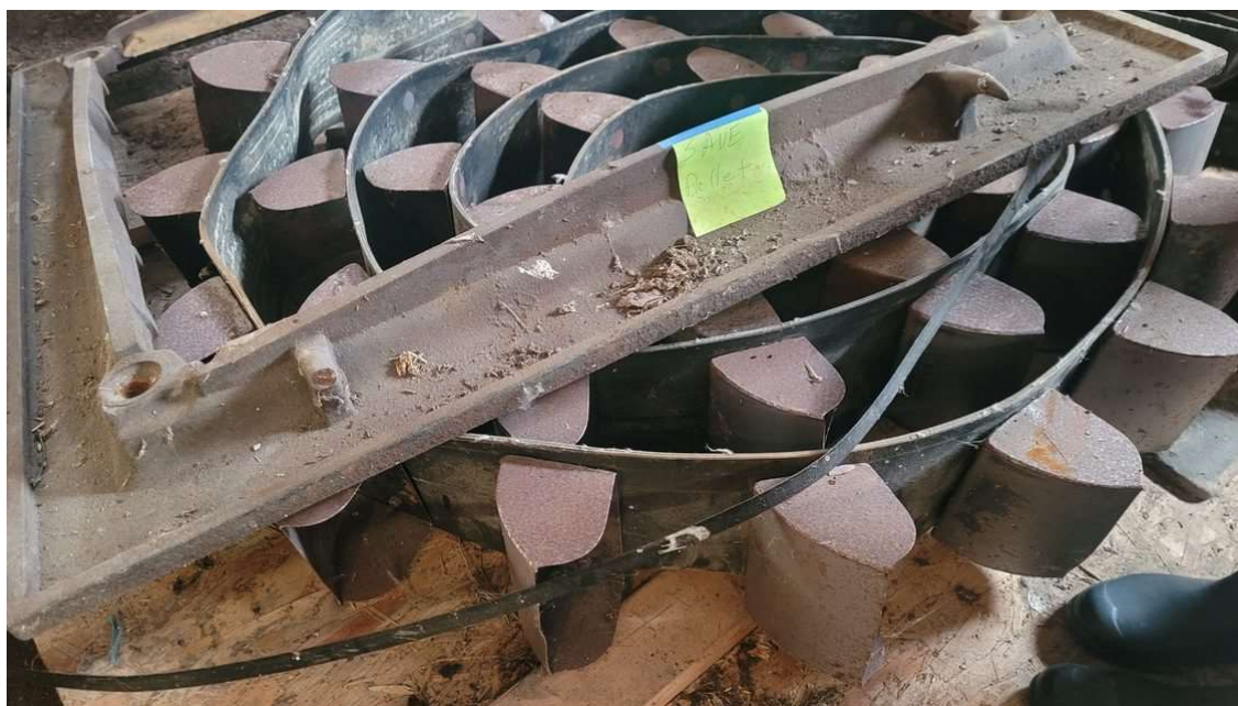
Grain elevator belt salvaged from the Teweles & Brandeis Grain Elevator in 2018. Currently stored offsite.
